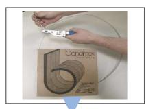
Cut off adequate band from roll 1/4" or 3/8" Bandimex band by opening the slot in the head of the tool with the cut off lefer at right angels to the tool. Thread the band through the slot and cut.
