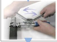
Depress locking pawl and tension clamp with forward strokes of the ratchet wrench.
