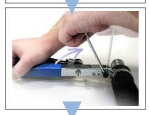
Cut off excess band by lifting cutter lever.
