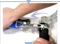
When sufficient tension has been applied, release locking pawl and rotate tool over object being clamped.
