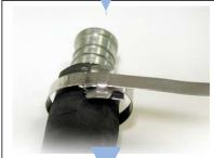
Form a clamp by threading the band through buckle and make a fold under the buckle.
