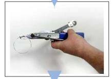
Insert tail of clamp into head of tool and slide into slot of winding mandrel.
